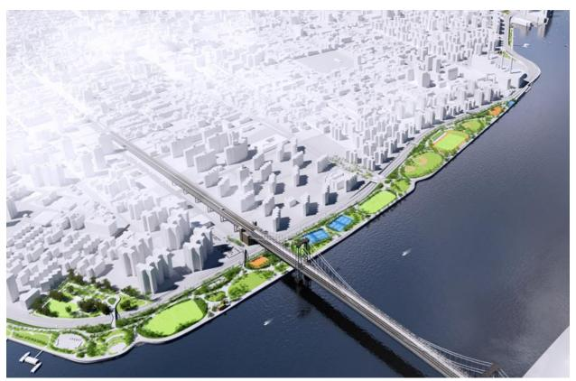
The East Side Coastal Resiliency project uses a series of berms, flood walls, flood gates and raised parklands to create a continuous 2.4-mile barrier to protect 110,000 residents of the Lower East Side in Manhattan from future coastal and tidal flooding
